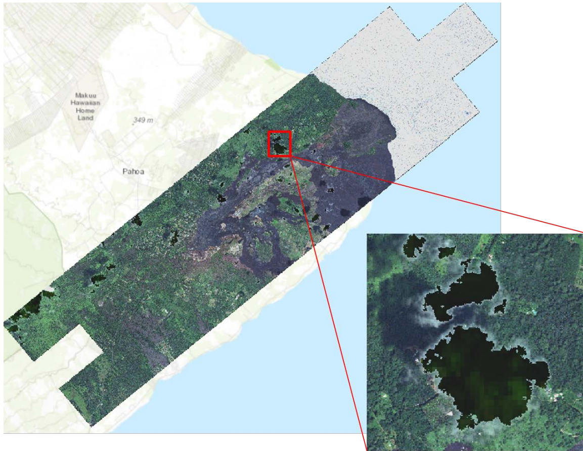
Figure 4: The Mosaic Operator set to First, the Mosaic Colormap Mode set to Match, and the Color Matching Method set to Match Histogram.
