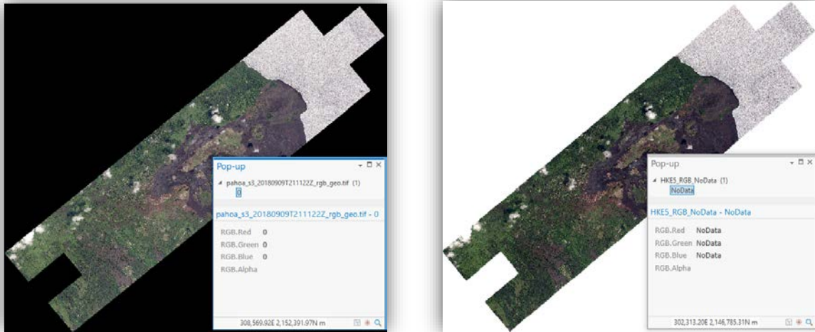
Figure 3: Digital Globe Imagery with background set at zero and with background set to NoData
