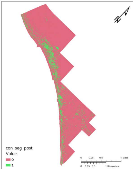
Figure 5: This is the resulting raster from the conditional statement, with 0 being non-damaged areas and 1 being damage
